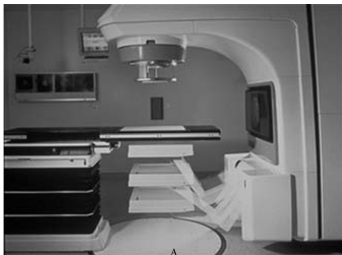
FIGURE 2 (A) Typical radiotherapy equipment. A patient is accurately positioned on the treatment table using side lasers. The head of the linear accelerator is above the treatment table, while below the treatment table one sees the electronic portal imaging device (mounted on a robot arm) that is used to verify the position of the patient relative to the treatment beam. The accelerator and table can rotate to allow targeting of a tumor from any direction. Photo courtesy of Varian Medical Systems, Palo Alto, CA. (B) The images made with the portal imager inherently have a poor image quality because of the high energy of the treatment beam. This is a portal image of a treatment in the pelvic area, where the black square is the treatment field.
