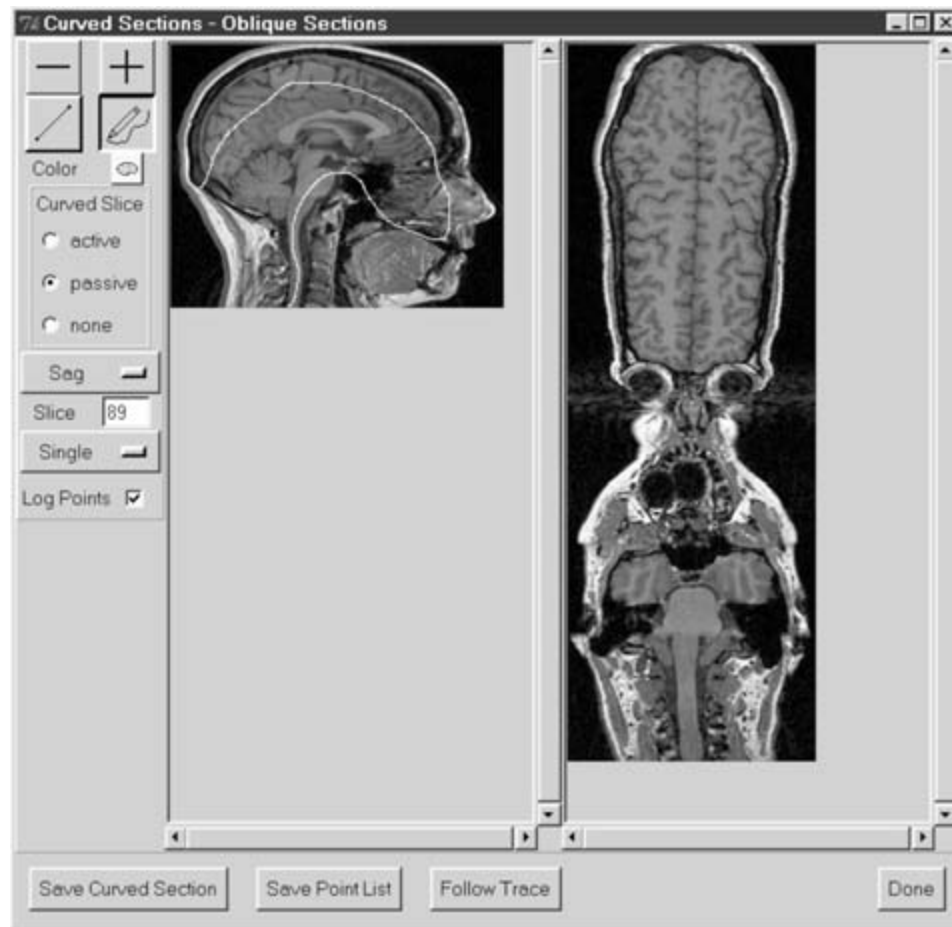
FIGURE 4 Tracing along an arbitrary path on an orthogonal image (top left) interactively generates and displays a curved planar image (right) sampled through the 3D volume image along that trace.
