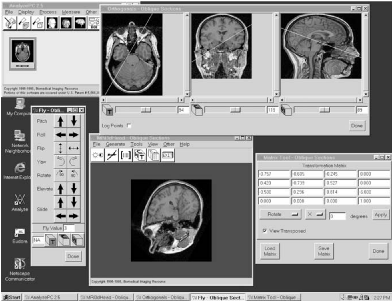
FIGURE 3 Arbitrarily oriented section (bottom center) cut obliquely through the 3D volume image can be interactively selected and computed. Interactive orientation is controlled by aeronautical maneuvers (pitch, roll, yaw, elevate options seen at right), with a graphical indication of the intersection of the oblique plane with orthogonal images (top row) used as orientation reference.
